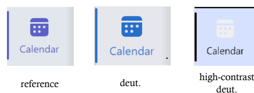
Figure 11. Reduced functionality in high contrast mode. In this instance, turning the calendar icon black would have helped to maintain functionality.
