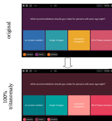
Figure 2: Screenshot processed with simulated CVD simulation [MOF09]. Contrast across UI components can often be reduced.
